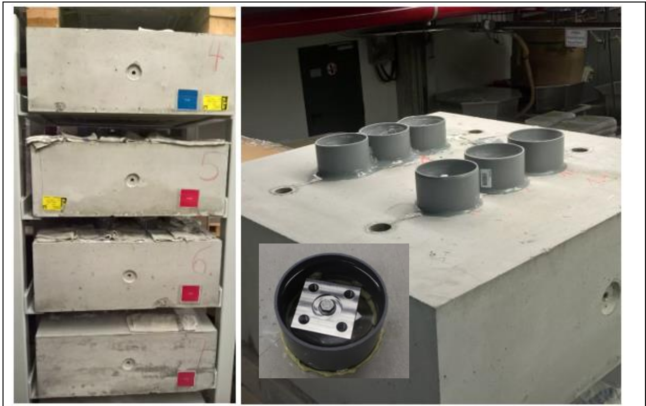
Figure 2.2.20.1.2.1.1 Storage in alkalinity or acid environment of the fasteners installed fasteners in concrete
