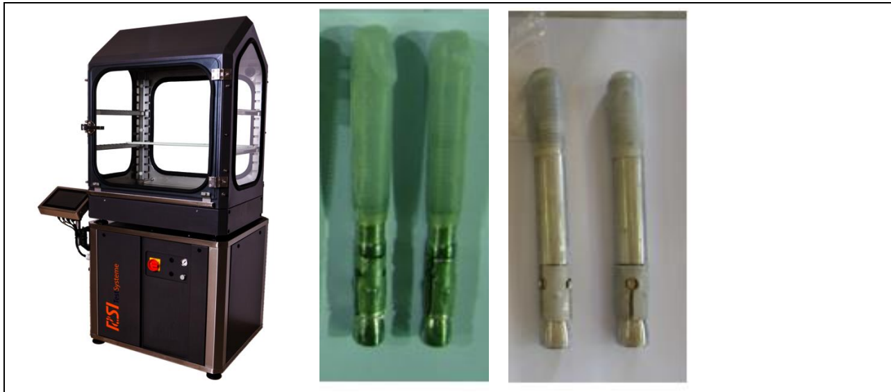
Figure 2.2.20.1.1.2.1 Storage in sulphurous environment and fasteners with sealed threads stored
